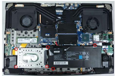
3.Unfasten six screws and pull out the battery, HDD module
