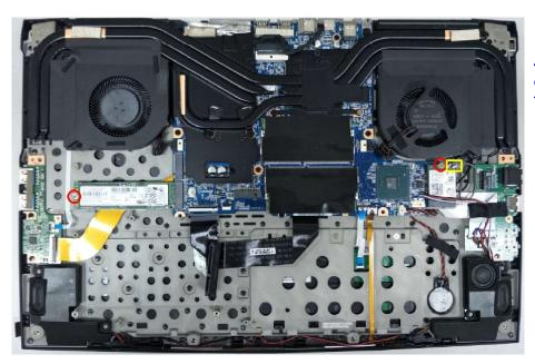
4. Unfasten two screws disconnect the wlan antenna. take out the SSD,WLAN
