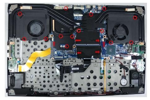
5.Unlock the RAM and take out the RAM. Unfasten fourteen screws of the FAN and the thermal module. Disconnect the cable of the Fan then remove them
